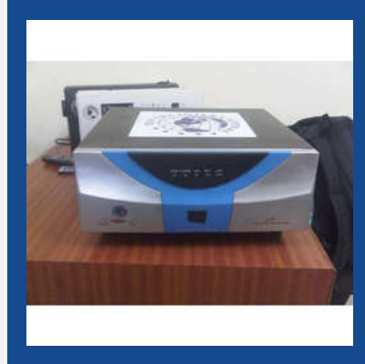
Solar Power Inverter
